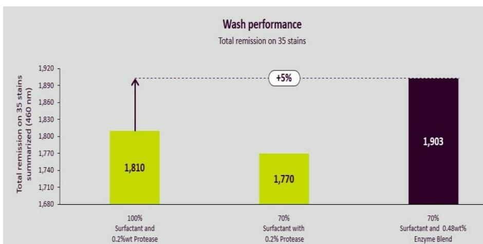
**Figure 1. After 30% reduction on surfactants, enzyme products could still deliver 5% performance increase<sup>14</sup>**
